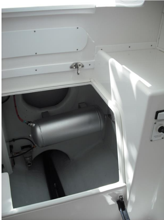
Holding Tank Seacock valve is accessible through the the steps inside the console.
