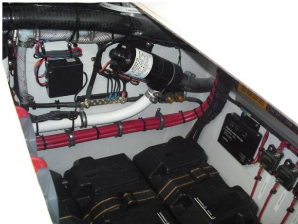
Macerator Pump is located inside the battery compartment
