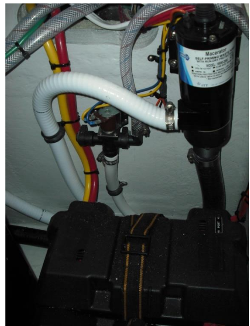
Holding tank seacock (**See Seacocks for open and closed positions)
