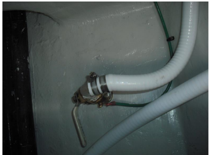
Holding tank seacock (**See Seacocks for open and closed positions)
