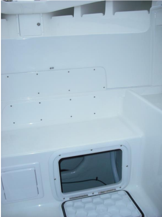
Holding Tank Seacock valve is accessible through the inspection hatch located on the steps inside the console.
