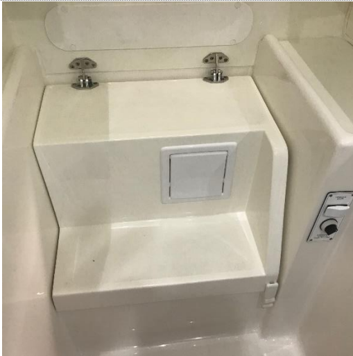
Holding Tank Seacock valve is accessible through the inspection hatch located on the steps inside the console.
