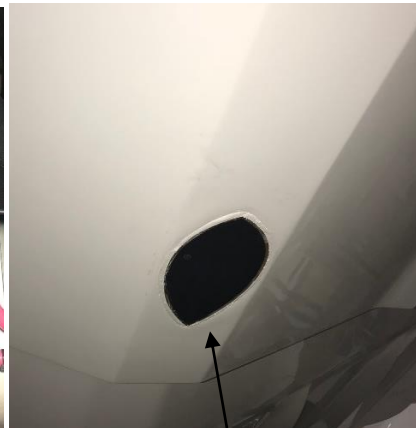
Transducer installed forward of the first hull step
