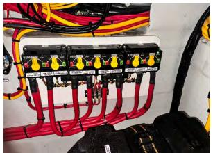
Figure 53 - Battery Switches inside the Battery Storage Compartment in the Console.
