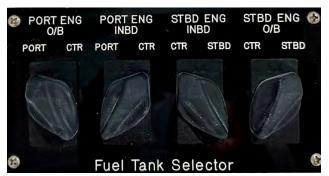
Figure 19 – Fuel Selector Panel for Four Engines
