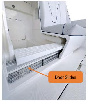
Figure 96 - Console Sliding Rails
