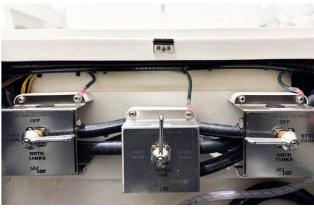
Figure 17- Manual Fuel Selector Valves for Triple Engine Configuration inside Bilge
