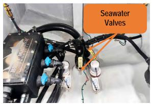
Figure 72 - Seawater Flush Pick-Up Valve at the Bilge Hatch.
