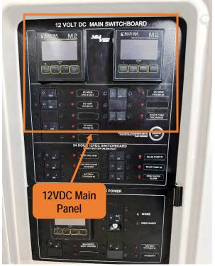
Figure 55 – 12VDC Main Distribution Panel.
