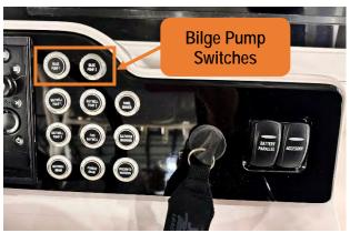
Figure 31 - Bilge Pump Switch Buttons.
