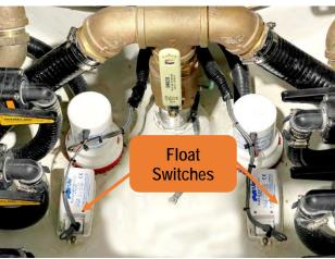
Figure 34 - Float Switches Inside the Bilge Hatch.
