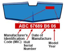
Figure 8 - Hull Identification Number Location.
