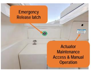
Figure 79 – Console Door Interior Emergency Release Latch & Actuator Access.
