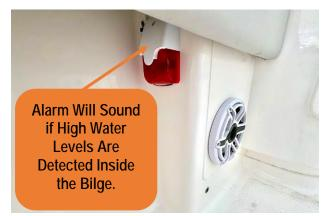
Figure 32 -Bilge Alarm at Beneath the Gunnel at the Starboard Aft Column.
