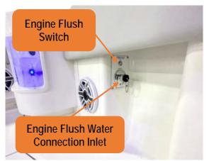
Figure 27 – Engine Flush System Switch on the Deck Port Side.
