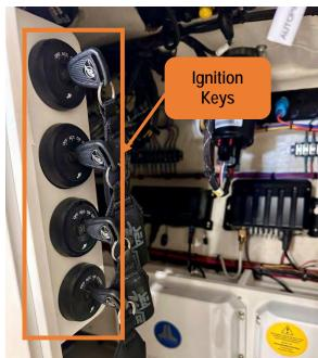
Figure 25 – Ignition Keys Location at the Main Rigging Electronic Access.
