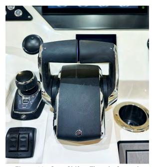
Figure 16 - Gear Shift & Throttle Control
