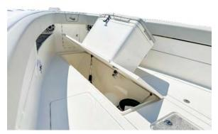
Figure 90 - Coffin Box and Hatch Actuator.
