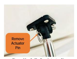
Figure 92 – Coffin Box Actuator Pin
