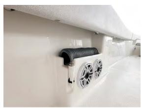
Figure 44 - Salt WaterWashdown Hose Coil at the Port Aft Cockpit Column.
