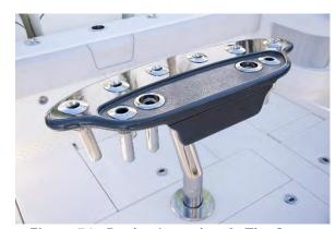
Figure 74 - Rocket Launcher At The Stern.
