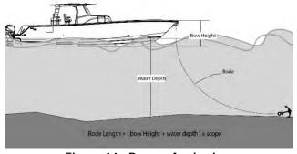
Figure 14 - Proper Anchoring
