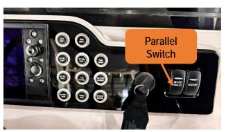
Figure 54 - Battery Parallel Switch on the Auxiliary Dash.
