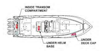
Figure 1 - ABYC Recommended Fire Extinguisher Locations for Boats under 40 Feet.
