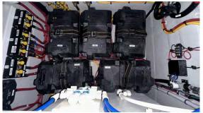
Figure 52 – Group 31 Batteries inside the Battery Compartment in the Console.
