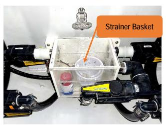
Figure 76 – Main FishboxStrainer inside the Bilge.
