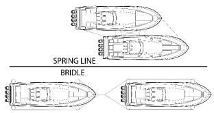
Figure 9 - Methods of Towing
