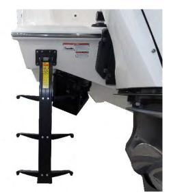
Figure 83 - Transom Tube Ladder at Port Side
