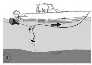
Figure 15 - Retrieve a Fouled Anchor with a Ball
