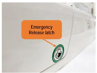
Figure 80 - Console External Emergency Release
