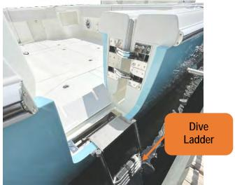
Figure 81 - Dive Hull Ladder at the Port Side.
