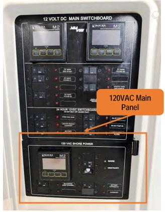
Figure 62 - 120VAC Main Distribution Panel with Shore Power Control inside the Console.
