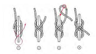
Figure 10 - Docking Belaying Knot
