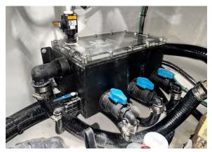
Figure 71 - Three Pumps Seachest
