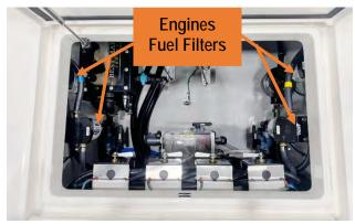
Figure 22 - Fuel Filters at Aft Bilge.
