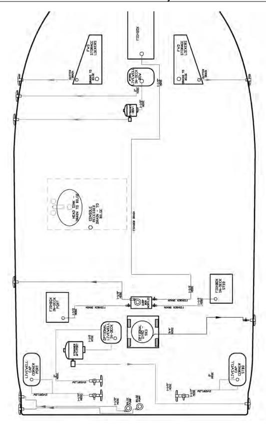
Diagram 22 -Hull Drainage & Plumbing Plan.
