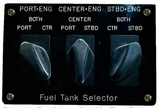
Figure 20 - Fuel Selector Panel for Three Engines.
