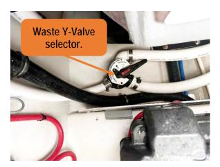
Figure 47 – Waste Y-Valve behind Console Stairs
