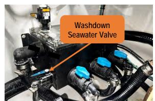
Figure 43 - Salt Water Wash Down Valve Located at the Forward Face of the Seachest.
