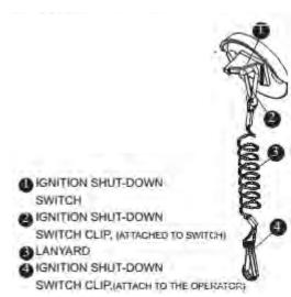
Figure 7 – Emergency Stop Switch.
