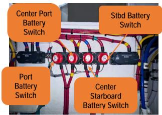
Figure 59 - Battery Switch below the Electronic Hatch Inside The Console.
