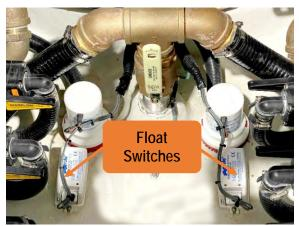
Figure 32 - Float Switches Inside The Bilge Hatch.
