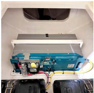
Figure 57 – Heavy Duty MLI 24/6000 Battery Inside The Battery Inverter Space In The Console.
