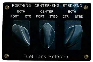
Figure 19 - Fuel Selector Panel Fo Three Engines.
