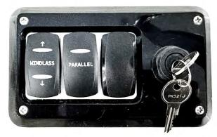
Figure 62 - Battery Parallel Switch On The Auxiliary Dash.
