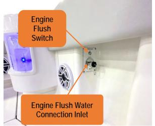
Figure 26 - Flushing System Switch On The Deck Port Side.
