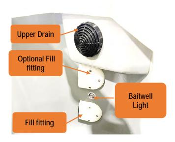
Figure 80 – Inside The Baitwell Tank System.
