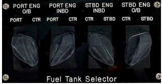
Figure 20 - Fuel Selector Panel For Four Engines
