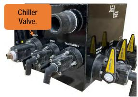
Figure 86 - Chiller Valve At The Forward Face Of The Port Seachest.
