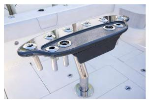
Figure 85 - Rocket Launcher At The Stern.
