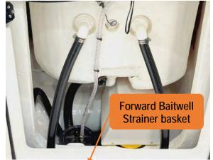
Figure 90 – Forward Baitwell Strainer Inside The Console.
