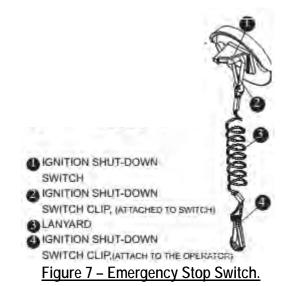
If an emergency arises and the engine must be shut down, a pull-on the cord to release the clip from the shut-off will shut off the engine.
