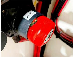
Figure 61 - Manual Battery Switch Turned On.
