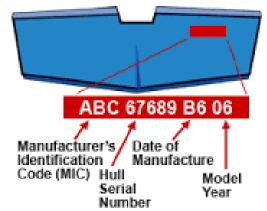
Figure 8 - Hull Identification Number Location.
