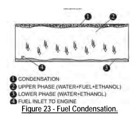
A partially full tank is not recommended because the void above the fuel allows air movement that can accumulate water through condensation as the air temperature moves up and down. This condensation
