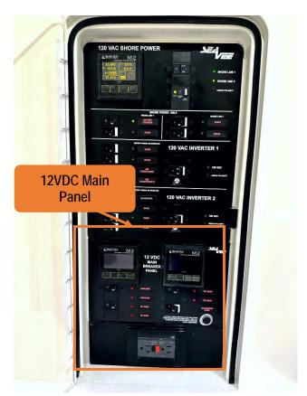
Figure 63 – 12VDC Main Distribution Panel.
