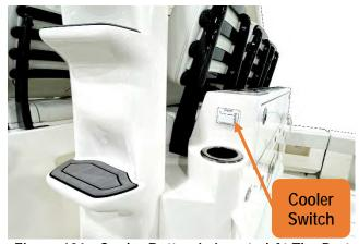
Figure 101 - Cooler Button Is Located At The Port Side Of The Aft Seat.
