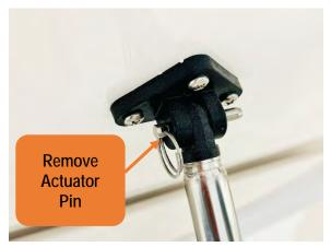
Figure 106 - Coffin Box Actuator Pin
