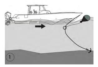
hanging in the ring, stop the boat, turn toward the anchor, and haul it in, bumping in and out of gear to ease the anchor handler's job.
