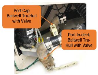
Figure 34 – Port Baitwell Tru-Hull Valve Located
