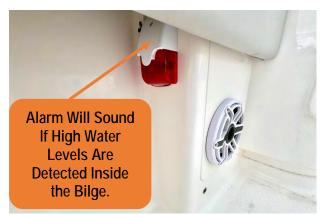
Figure 33 -Bilge Alarm At Beneath The Gunnel At The Starboard Aft Column.
