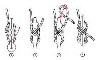
Figure 10 - Docking Belaying Knot
