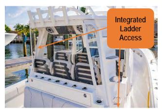
Figure 108 - Integrated Stairs for Second Station.
