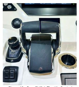
Figure 18 - Gear Shift & Throttle Control
