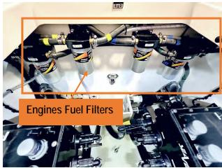
Figure 22 - Fuel Filters At Aft Bilge Hatch.
