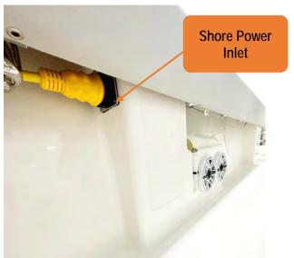
Figure 71 - Shore Power Inlet At The Starboard Middle Column.
