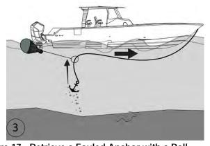
Figure 17 - Retrieve a Fouled Anchor with a Ball
