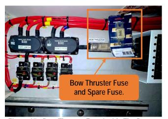
Figure 87 - Bow Thruster Fuse Inside The Battery Hatch In The Console.
