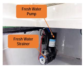
Figure 40 - Fresh WaterPump Inside The Starboard Auxiliary Bilge Hatch.
