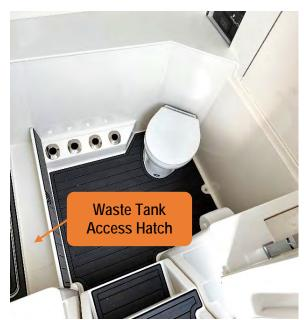
Figure 50 - Access Hatch For Waste Tank Below The Shelf Keeper.
