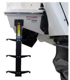
Figure 96 - Transom Tube Ladder At Port Side
