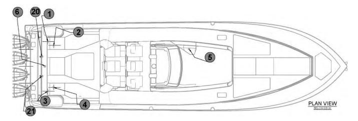
The liner, cockpit, and console are shown for reference. All thru hulls are at the hull bottom.
