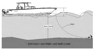
Figure 16 - Proper Anchoring
