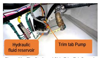
Figure 29 – The Starboard Side Trim Tab Pump is
