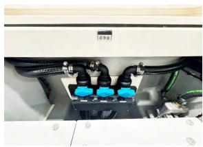
Figure 84 – Seachest Manifold Located at the Auxyliary Machinery compartment
