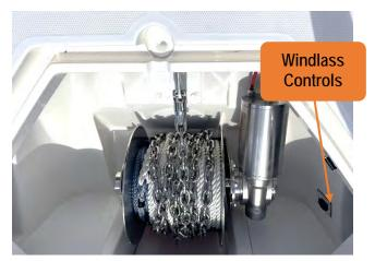
Figure 13 – Drum Style Windlass & Button Inside
