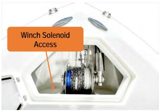
Figure 15 - Windlass/Winch Solenoid Access.
