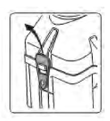
Unscrew the cap and check the fluid level in the reservoir; fill ONLY with SAE 0W-30 Synthetic Power Steering Fluid if necessary.
