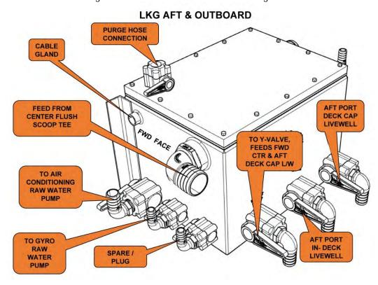
Diagram 38 - Seachest Starboard Side Configuration.
