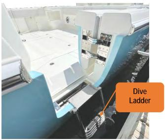
Figure 94 - dive hull ladder at the port side
