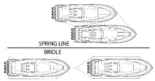
Figure 9 - Methods Of Towing
