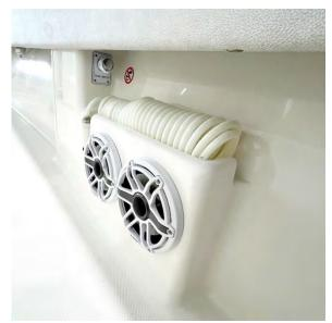
Figure 38 - Fresh Water Wash Down Hose In The Aft Starboard Cockpit.
