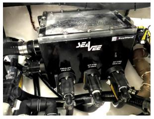
Figure 80 - Seachest Starboard Side.
