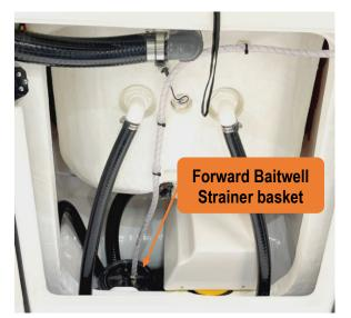
Figure 88 – Forward Baitwell Strainer Inside The Cabin.
