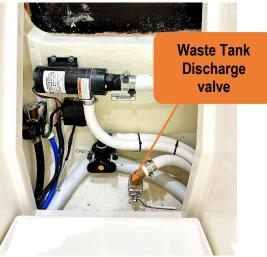
Figure 35 – Overboard Waste Tank Discharge Valve Is Located Under The Cabin's Stairs.
