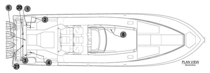
The liner, cockpit, and cabin are shown for reference. All thru hulls are at the hull bottom. Diagram 11 -Thru-Hull Fittings Below Deck Plan View.
