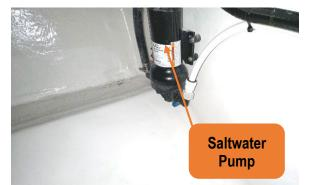
Figure 47 – Saltwater Pump At The Starboard Side Of The Auxiliary Machinery Space
