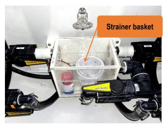
Figure 86 – Main Fish Box Strainer Inside The Bilge.
