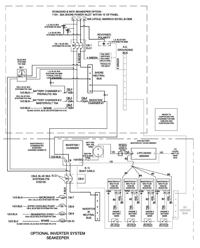
Diagram 28 – 120VAC/50Amp Main Electrical Distribution Panel With Seakeeper Wiring Diagram 50 Amp Shore Power And Inverter
