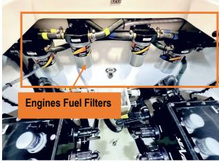
Figure 20 - Fuel Filters At Aft Bilge Hatch.
