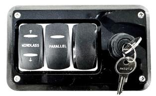
Figure 61 - Battery Parallel Switch On The Auxiliary Dash.
