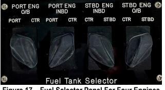
Figure 17 – Fuel Selector Panel For Four Engines
