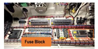
Figure 68 Electronics Fuse Blocks In The Electrical Rigging Compartment Inside The Cabin.
