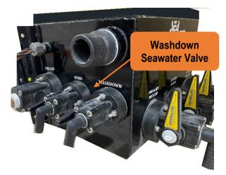
Figure 46 - Salt Water Wash Down Valve Located At The Forward Face Of The Starboard Seachest.
