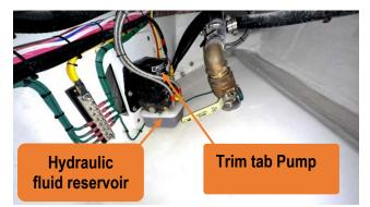
Figure 27 – The Starboard Side Trim Tab Pump Is Located Inside The Auxiliary Machinery Hatch.
