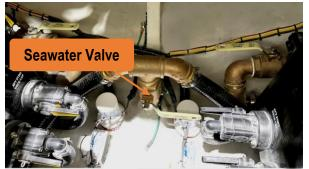
Figure 81 - Seawater Flush Pick-Up Valve At The Bilge Hatch.
