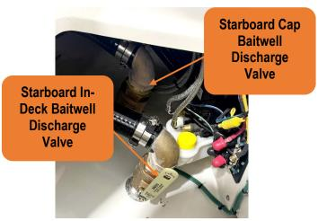
Figure 34 – Starboard Baitwell Discharge Valve Located At The Port Auxiliary Bilge.
