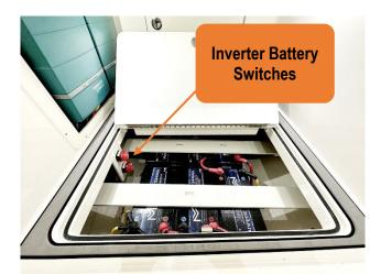
Figure 59 - Inverter Battery Switches For Inside The Inverter Battery Space In The Forward Cabin.
