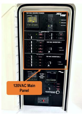
Figure 69 - 120VAC Main Distribution Panel With Shore Power Control Inside The Cabin.
