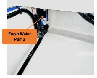
Figure 39 - Freshwater Pump Inside The Starboard Auxiliary Bilge Hatch.
