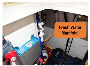
Figure 40 - fresh water manifold is accessed from main rigging and electronics access hatch.
