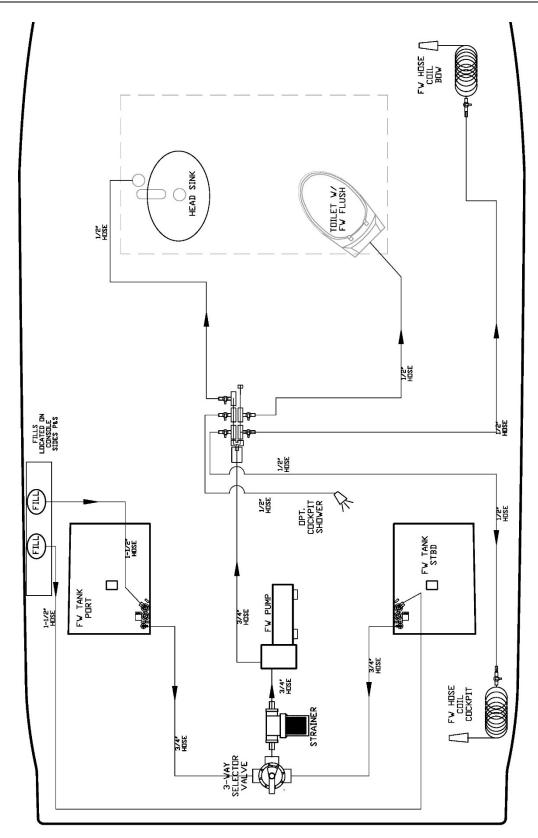
Diagram 18 - Fresh Water System Diagram.
