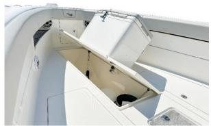
Figure 102 – Coffin Box And Hatch Actuator.
