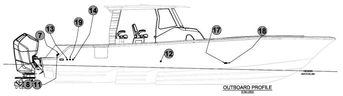
Diagram 12 - Thru Hull Fittings Outboard Starboard Side.
