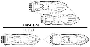
Figure 7 - Methods Of Towing
