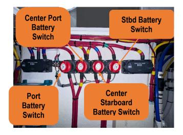
Figure 58 - Battery Switch below the Electronic Hatch Inside The Cabin.
