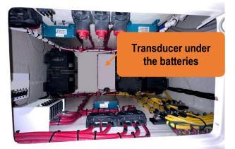
Figure 72 - Transducer Location Inside The Battery Hatch In The Electronics Compartment.
