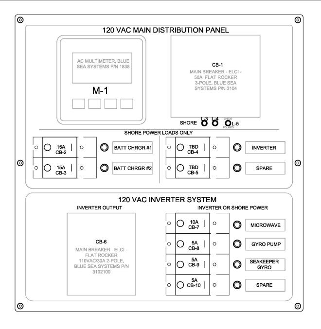
Diagram 27 – 120VAC/50Amp Main Electrical Distribution Panel With Seakeeper 50 Amp Shore Power And Inverter
