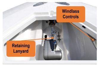
Figure 10 – Conventional Windlass Inside The Anchor Hatch.
