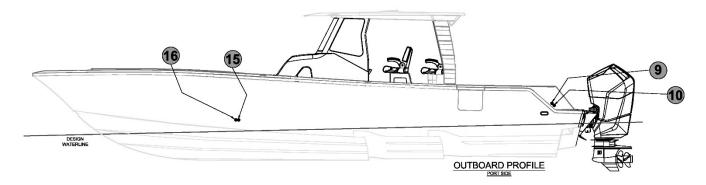
Diagram 13 -Thru-Hull Fittings Outboard Port Side.
