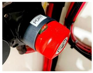
Figure 60 - Manual Battery Switch Turned On.
