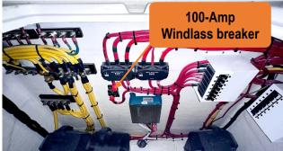
Figure 66 - 50-Amp DC Breakers Inside The Battery Hatch In The Cabin.
