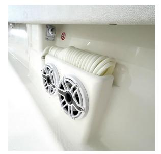
Figure 37 - Fresh Water Wash Down Hose In The Aft Starboard Cockpit.
