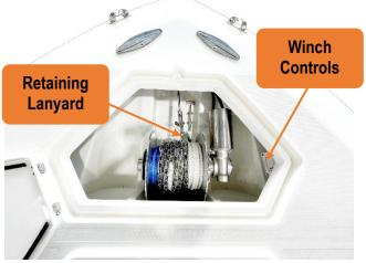
Figure 11 – Drum Style Windlass & Button Inside The Anchor Hatch
