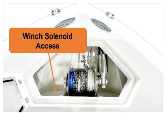
Figure 12 – Windlass/Winch Solenoid Access.
