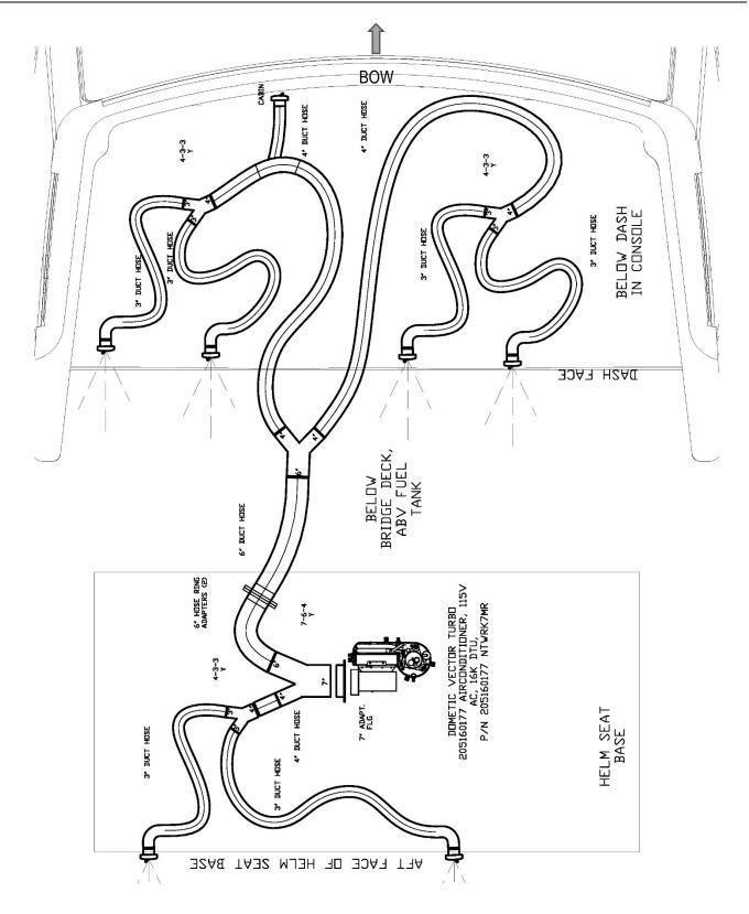
Diagram 21 - Air Conditioning System Diagram In The Helm.
