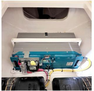
Figure 56 – Heavy Duty MLI 24/6000 Battery Inside The Battery Inverter Space In The Cabin.
