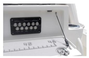
Figure 77 - Auxiliary Pump Panel At The Aft Seat.
