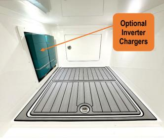
Figure 57 – Optional Inverter Chargers in the Forward Port storage area.
