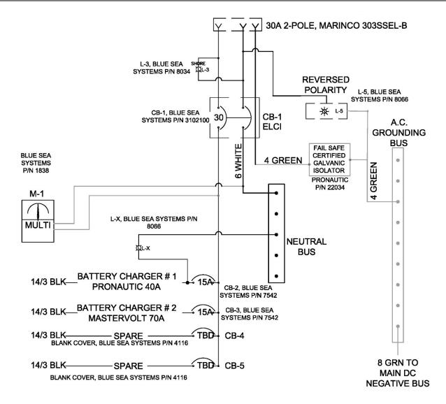
Diagram 26 -120VAC/30AMP Main Electrical Distribution Panel Wiring Diagram Standard Without Seakeeper Option – NO INVERTERS.
