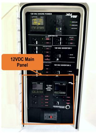
Figure 62 – 12VDC Main Distribution Panel.
