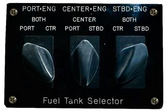
Figure 18 - Fuel Selector Panel Fo Three Engines.
