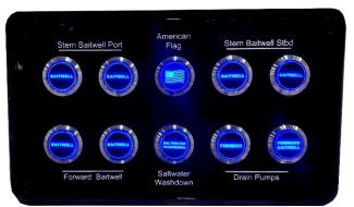
Figure 87 - auxiliary pump switch panel.
