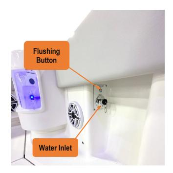
Figure 24 - Flushing System Switch On The Deck Port Side.
