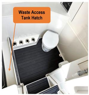
Figure 49 - Access Hatch For Waste Tank Below The Shelf Keeper.
