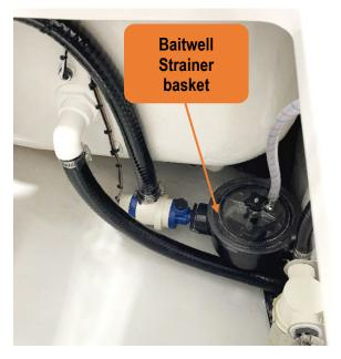
Figure 89 – Port In-Deck Baitwell Strainer Inside The Port Auxiliary Bilge Compartment.
