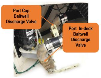
Figure 33 – Port Baitwell Discharge Valve Located At The Port Auxiliary Bilge.
