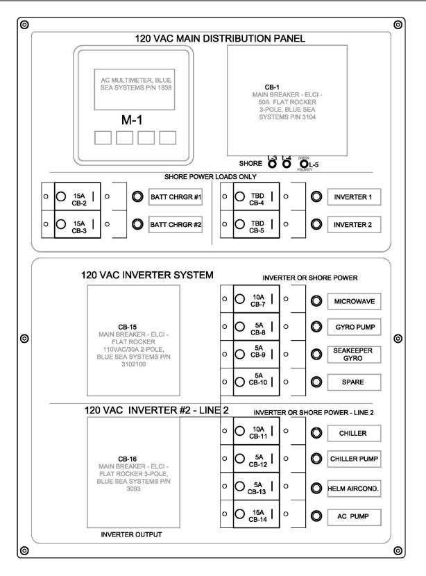
Diagram 29 - 120VAC/50Amp Main Electrical Distribution Panel With Seakeeper & Air Conditioning 50 Amp Shore Power And Two Inverters
