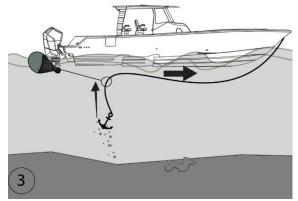
Figure 15 - Retrieve A Fouled Anchor With A Ball
