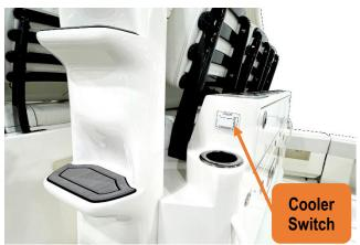
Figure 99 - Cooler Button Is Located At The Port Side Of The Aft Seat.
