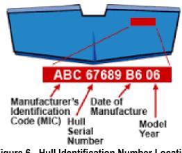
Figure 6 - Hull Identification Number Location.
