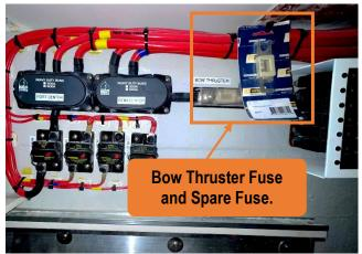
Figure 85 - Bow Thruster Fuse Inside The Battery Hatch In The Cabin.
