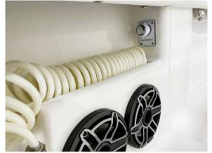
Figure 45 - Saltwater Washdown Hose Coil At The Port Aft Cockpit Column.
