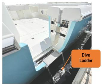
Figure 92 - dive hull ladder at the port side
