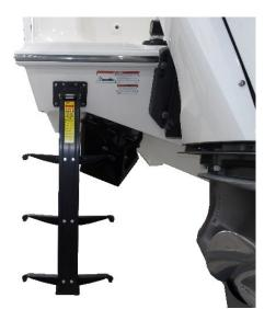
Figure 94 - Transom Tube Ladder At Port Side
