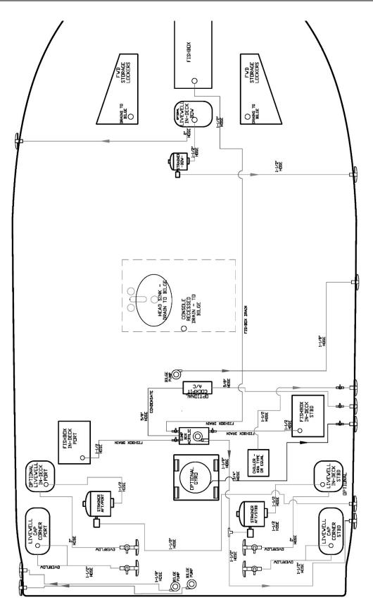
Diagram 17 -Hull Drainage & Plumbing Plan.
