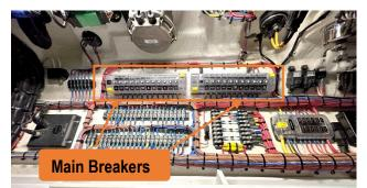
Figure 65 – 12VDC Main Breakers Inside The Electrical Rigging Area In The Restroom.
