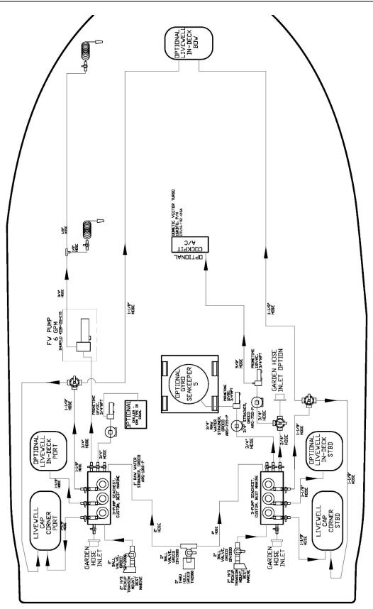
Diagram 19 - Raw Water System Diagram.
