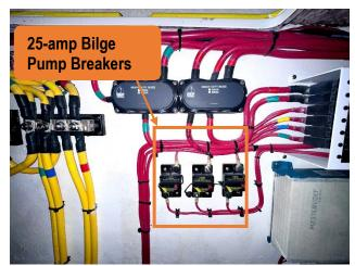
Figure 64- -Bilge And Windlass Breakers Inside The Battery Hatch In The Cabin.
