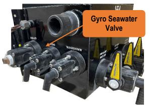
Figure 52 - Gyro Seawater Valve At The Forward Face Of The Starboard Seakeeper.
