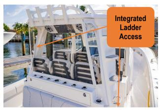
Figure 104 – Integrated Stairs for Second Station.
