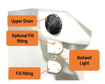
Figure 79 – Inside The Baitwell Tank System.
