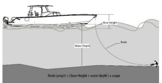
Figure 14 - Proper Anchoring
