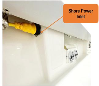
Figure 70 - Shore Power Inlet At The Starboard Middle Column.
