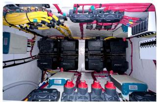
Figure 55 – Group 31 Batteries Inside The Battery Compartment In The Cabin.
