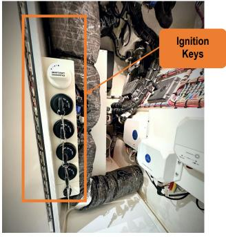
Figure 23 – Ignition Keys Location At The Main Rigging Electronic Access.
