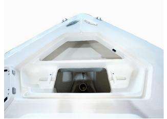
Figure 9 – Forward Molded Storage For Danforth/ Fluke Style Anchor.
