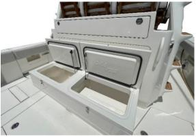
**Figure 95 - Electric Sliding Cooler.** An electric sliding dual cooler provides seating and
