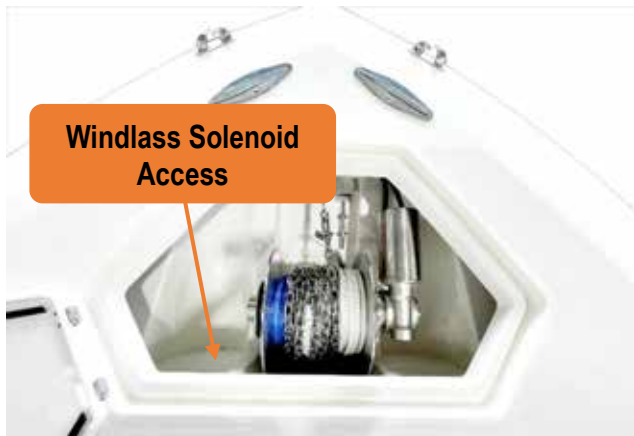
Figure 15 - windlass solenoid access.
