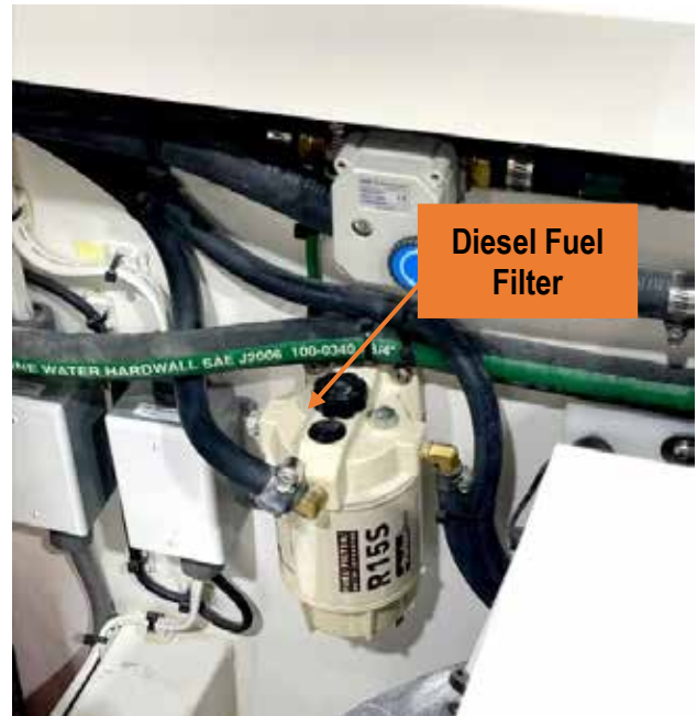
Figure 73 - diesel fuel filter inside the aft auxiliary machinery hatch.
