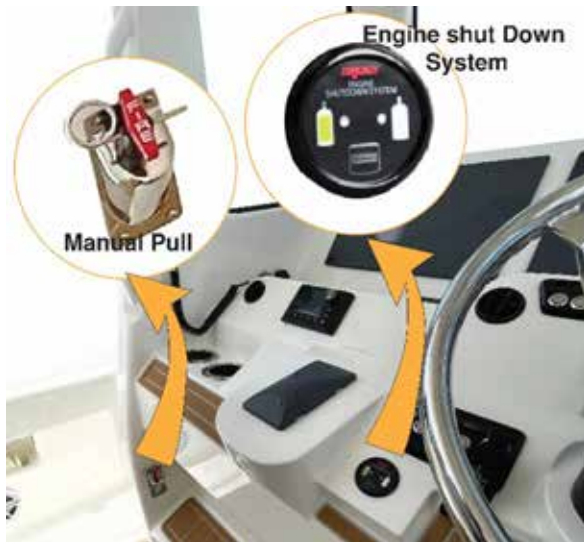
Figure 4 - manual pull & engine shut down system at the helm.
