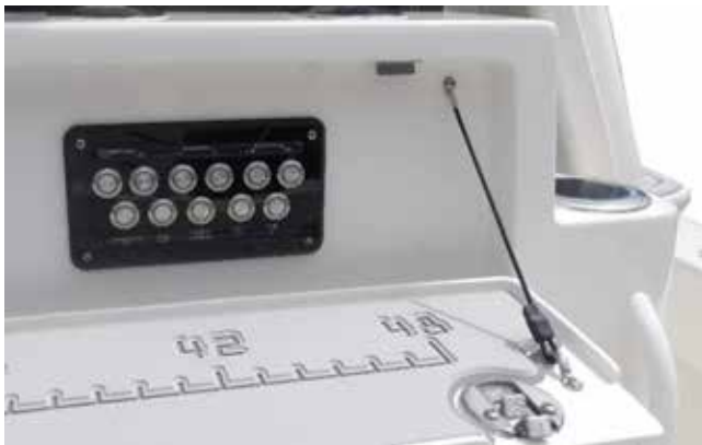
Figure 79 - auxiliary pump panel at the aft seat.
