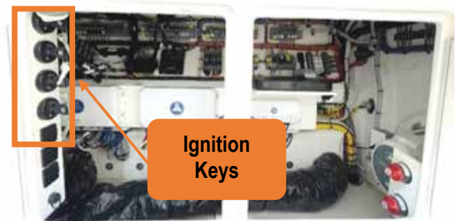
Figure 25 – ignition keys location at the main rigging electronic access.
