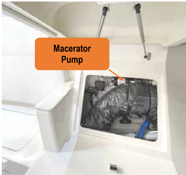
Figure 50 – macerator pump access hatch behind cabin stairs.
