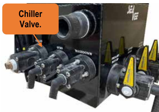
Figure 88 - chiller valve at the forward face of the starboard seachest.
