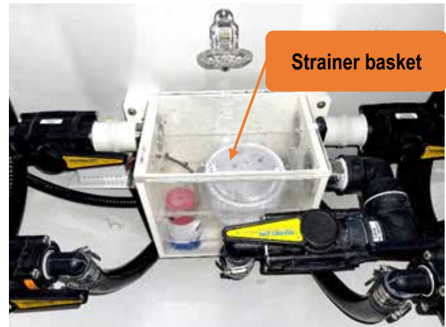
Figure 90 – main fish box strainer inside the bilge.
