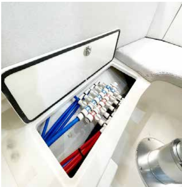
Figure 40 - fresh water manifold is accessed from under the cabin port seat hatch.
