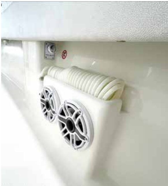
Diagram 18 - Fresh water wash down hose in the aft starboard cockpit.
