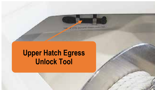
Figure 96 – cabin unlock tool inside the anchor hatch.
