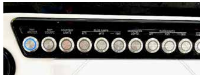
Figure 76 - blue lighting indicating navigation lights mode ON.
