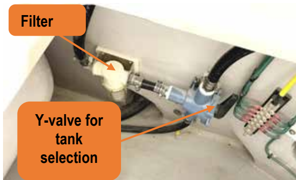
Figure 43 – Fresh water pump filter inside the port auxiliary bilge.
