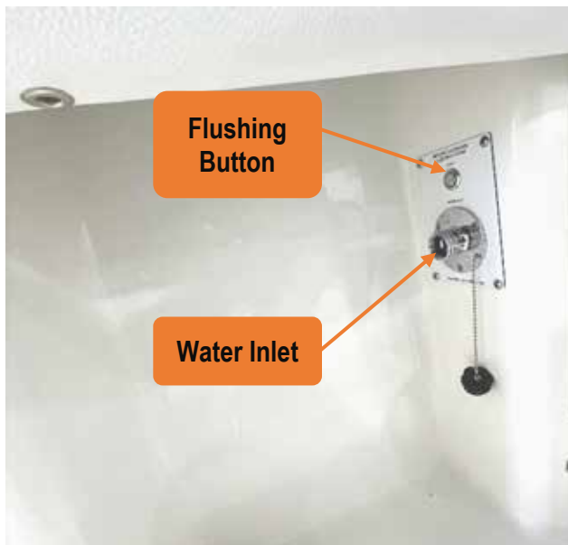
Figure 26 - reverso flushing switch on the deck - starboard side.
