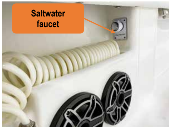
Figure 47 - saltwater washdown hose coil and faucet at the port aft cockpit column.
