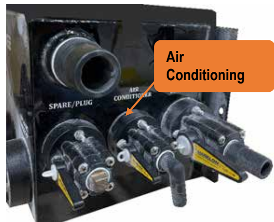
Figure 55 - air conditioning valve at the forward face of the port seachest.
