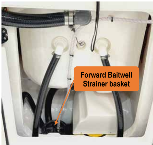
Figure 92 – forward baitwell strainer inside the cabin.
