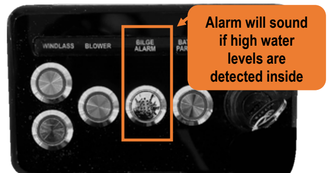
Figure 31 -bilge alarm at the auxiliary dash switch panel.
