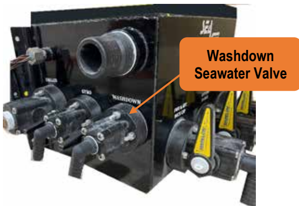
Figure 48 - salt water wash down valve located at the forward face of the starboard seachest.
