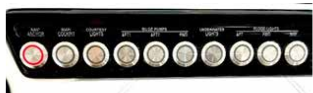
Figure 77 - red lighting indicating anchor light mode ON.
