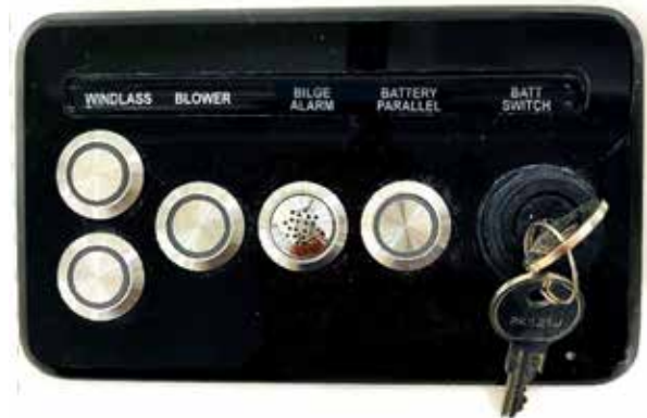
Figure 61 - battery parallel switch on the auxiliary dash
