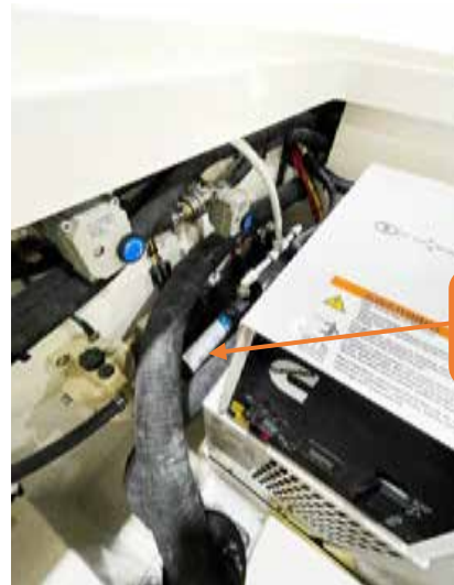
Figure 49 – saltwater pump at the starboard side of the auxiliary machinery space
