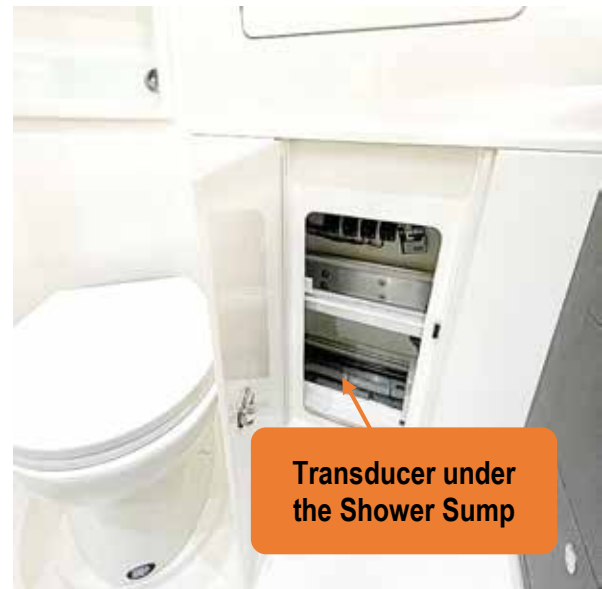
Figure 74 - transducer location inside the battery hatch in the toilet.
