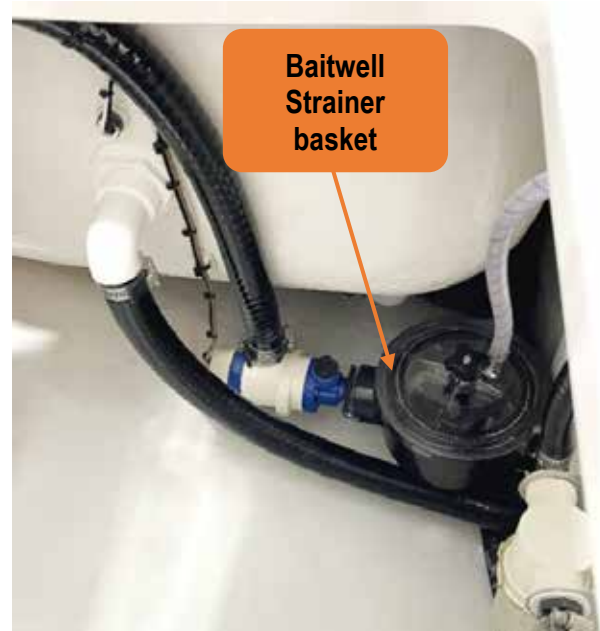
Figure 93 – port in-deck baitwell strainer inside the port auxiliary bilge compartment.
