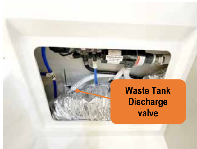
Figure 37 – overseas waste tank discharge valve is located under the cabin's stairs.
