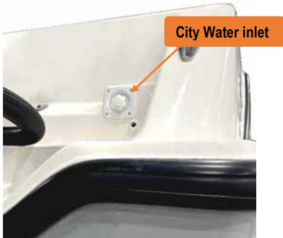
Figure 42 - fresh water inlet at the starboard side of the outside stern deck.
