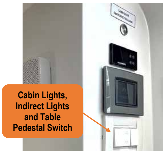
Figure 78 - cabin light control panel at the cabin entrance.
