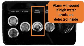
Figure 31 -bilge alarm at the auxiliary dash switch panel.
