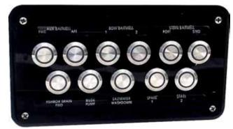
Figure 91 - auxiliary pump switch panel.
