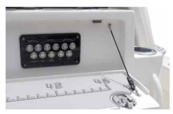
Figure 79 - auxiliary pump panel at the aft seat.
