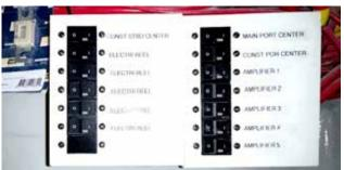
Figure 67 - 50-amp DC breakers inside the battery hatch in the cabin.
