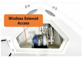
Figure 15 - windlass solenoid access.
