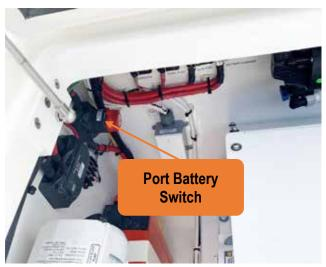
Figure 59 - battery switch for port and starboard
