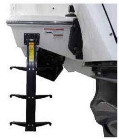
Figure 102 - transom tube ladder at port side
