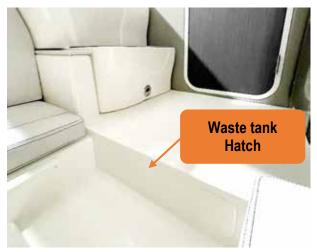
Figure 51 - access hatch for waste tank location.
